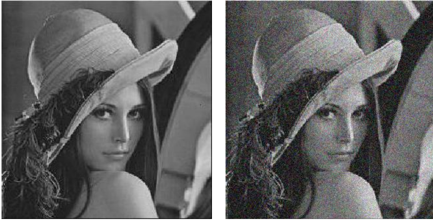
Figure 1.6 (a) clean image (b) image with Gaussian noise, with standard deviation \sigma = 25 , SNR=5.64dB.
