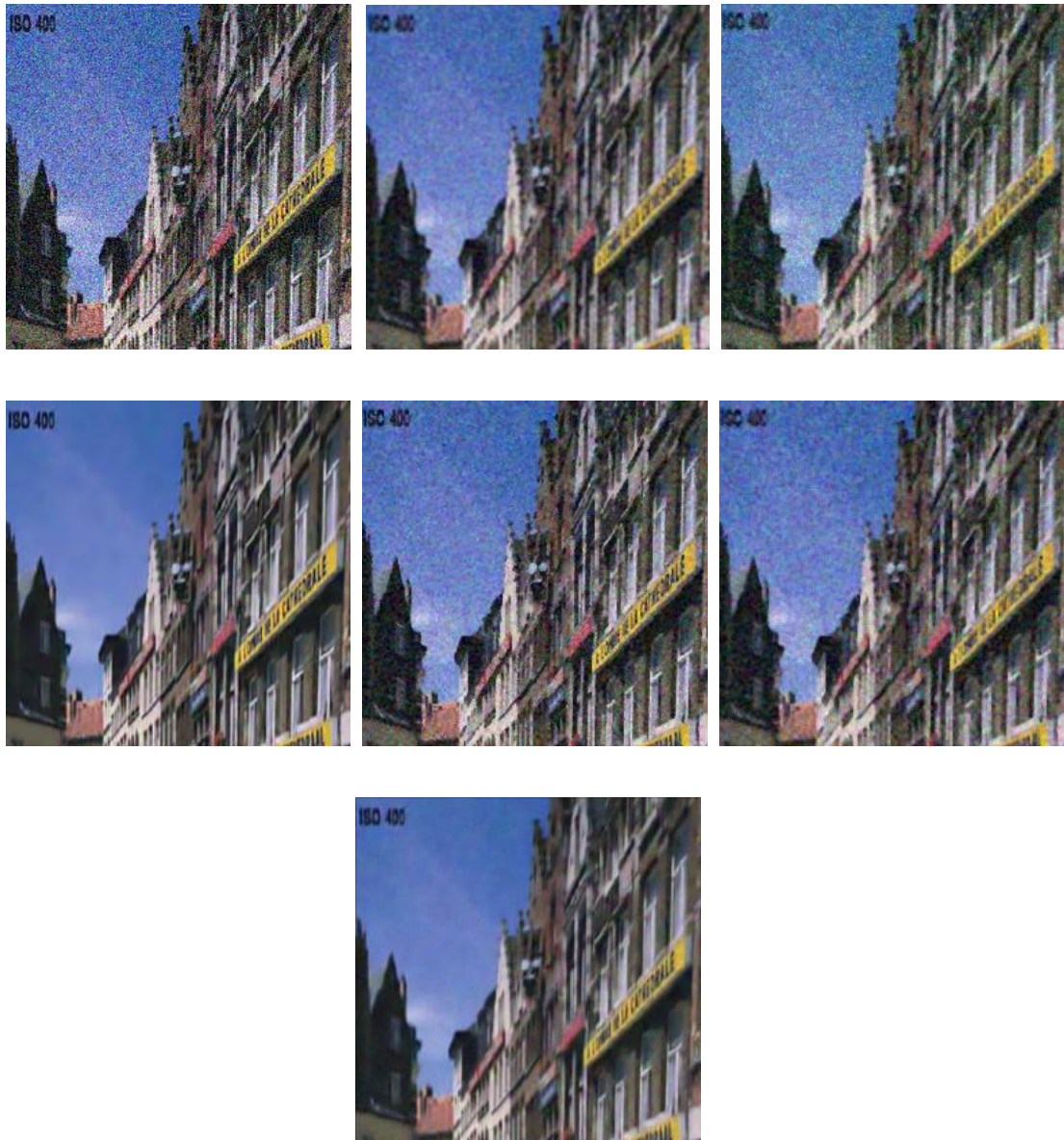
Figure 5.10: Denoised Cafe images obtained with different filters while the input to each filter has the same Level of noise (A) with Gaussian noise \sigma=30 , (B) FPGA, (C) SADA, (D)RICMG, (E) FFNRIC, (F) DBFIR, (G) the proposed method
