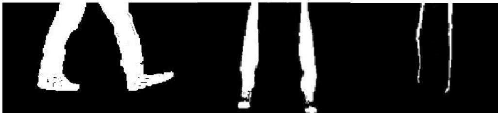
Figure 5(a). Connected pixel of lower part in binary image
