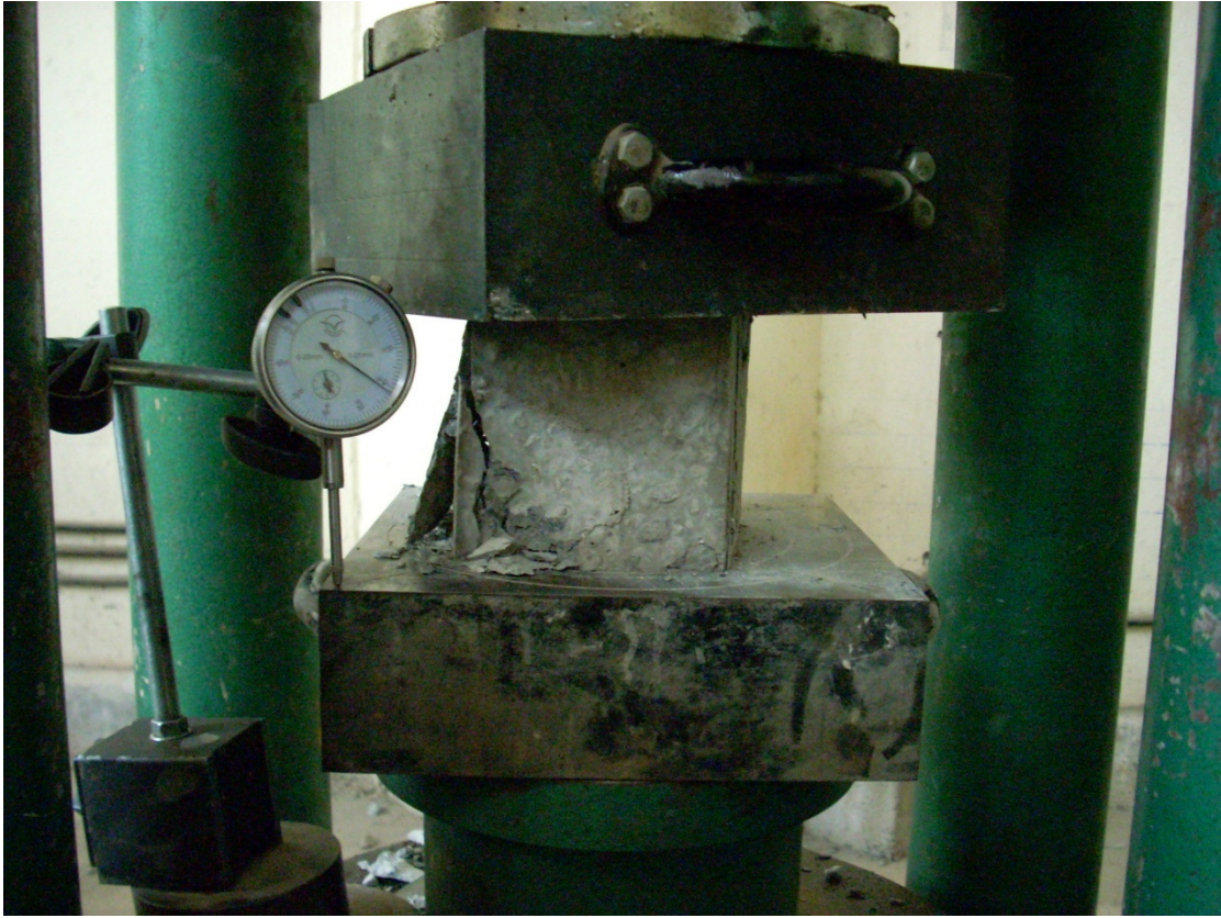
Fig. 3.3 Experimental setup for compression test
