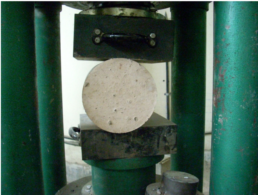
Fig. 3.6 Experimental setup for split tension test.
