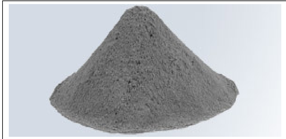
Fig. 2.14. As produced silica fume. This is what the material looks like after it is collected.
