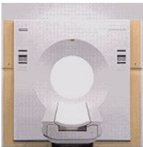
Outside view of modern CT system showing the patient table and CT scanning patient aperture
