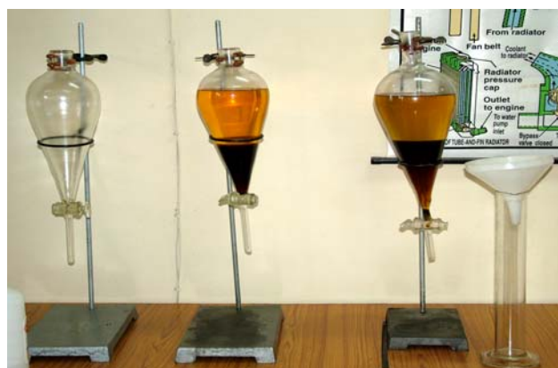
Fig 8.2 separations of biodiesel and glycerol taken place by the help of gravity in the separation funnel, as can be seen the black part is the settled part of glycerol.
