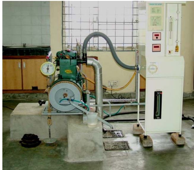
Fig 10.4: Kirloskar AV1/TV1/SV1/AK65 water cooled Diesel Engine Set up
