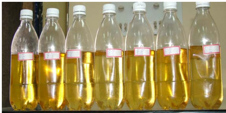
Fig 8.5- Of the samples which form different layers and they are partially miscible
