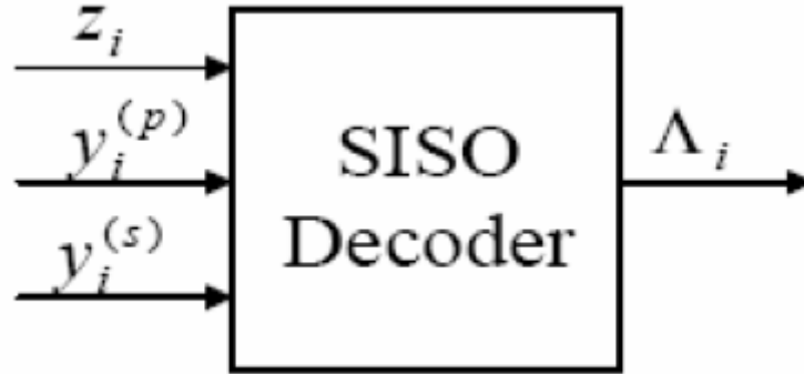
Figure 3.4 Soft-input soft-output module: z_i , the a priori values for information bits, y_i^{(p)} the parity observations, y_i^{(s)} and \Lambda_i the a posteriori values
