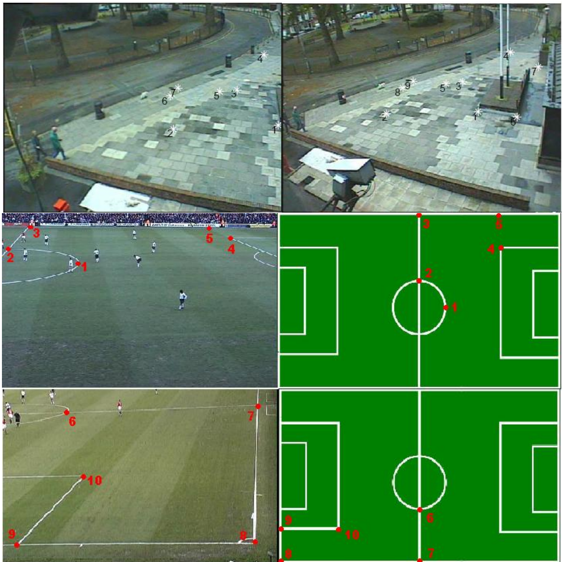
Figure 3.1 Example of landmark points gathered by a survey of the surveillance region
