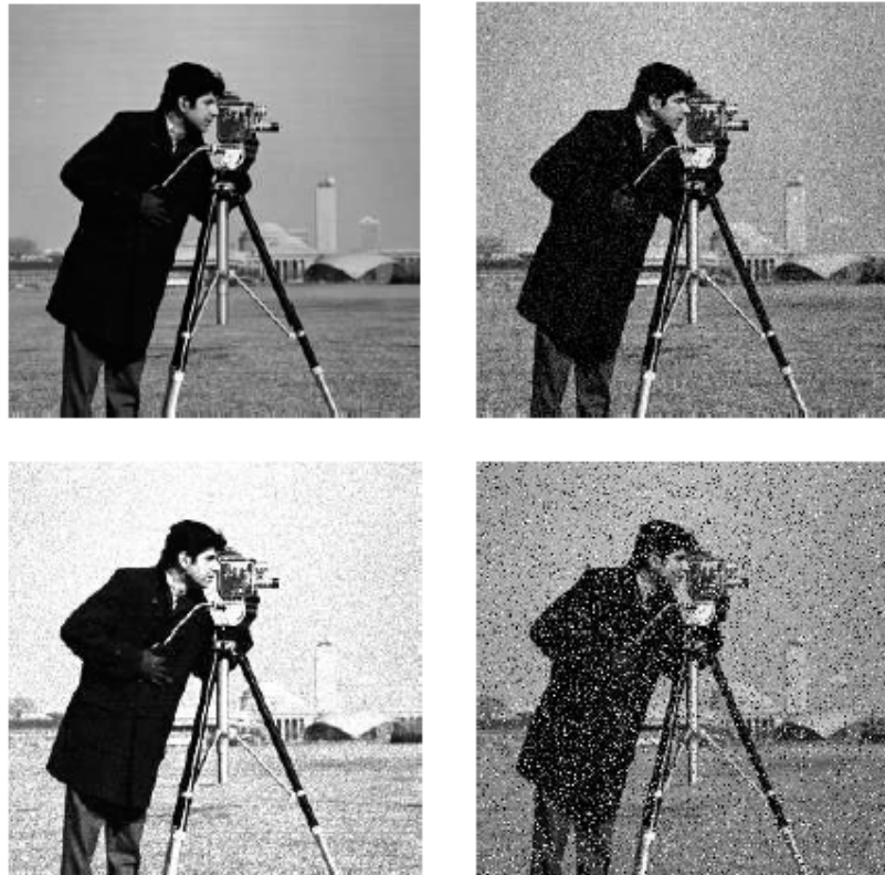
Figure 2.6: Different types of noise: (a) original image; (b) additive noise; (c) multiplicative noise; (d) impulse noise.
