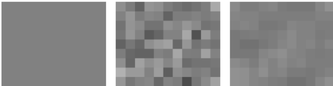
Figure 2.8: Application of the 3X3 box filter: (a) original; (b) noisy; (c) filtered.
