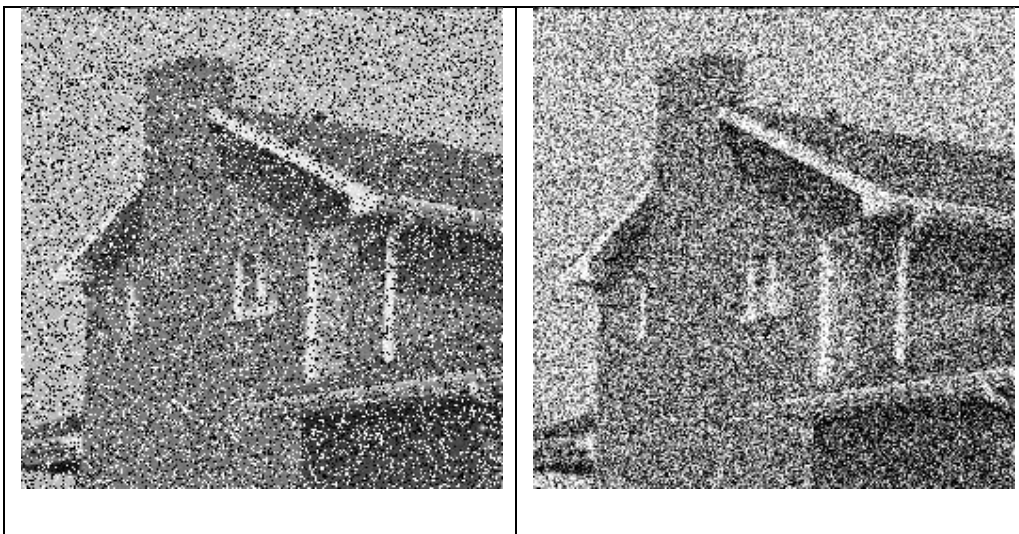
Fig.5.47 Red house with high impulse noise Fig5.50 Red house with high random noise
