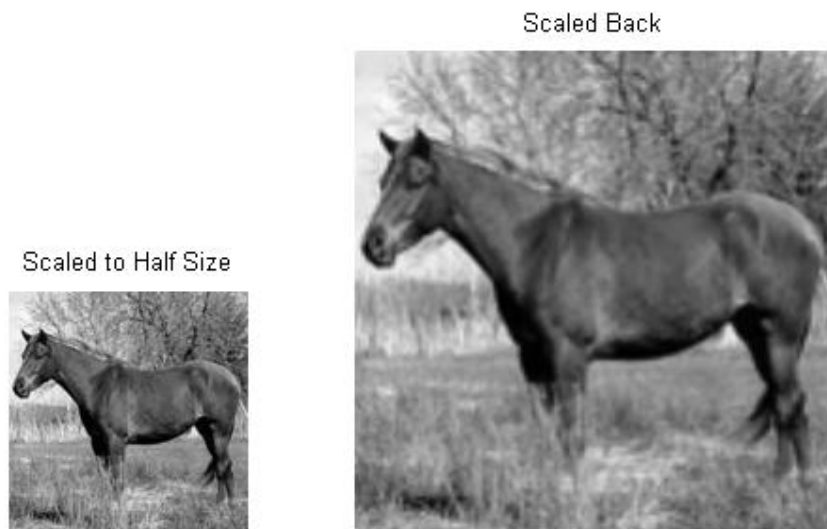
Figure 14(a): 0.5x Scaled image of “Horse” and 14(b): Scaled-back image to original size, showing noticeable loss of finer details.
