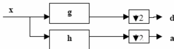
Figure B2.1: Splitting of the signal x into two parts.
