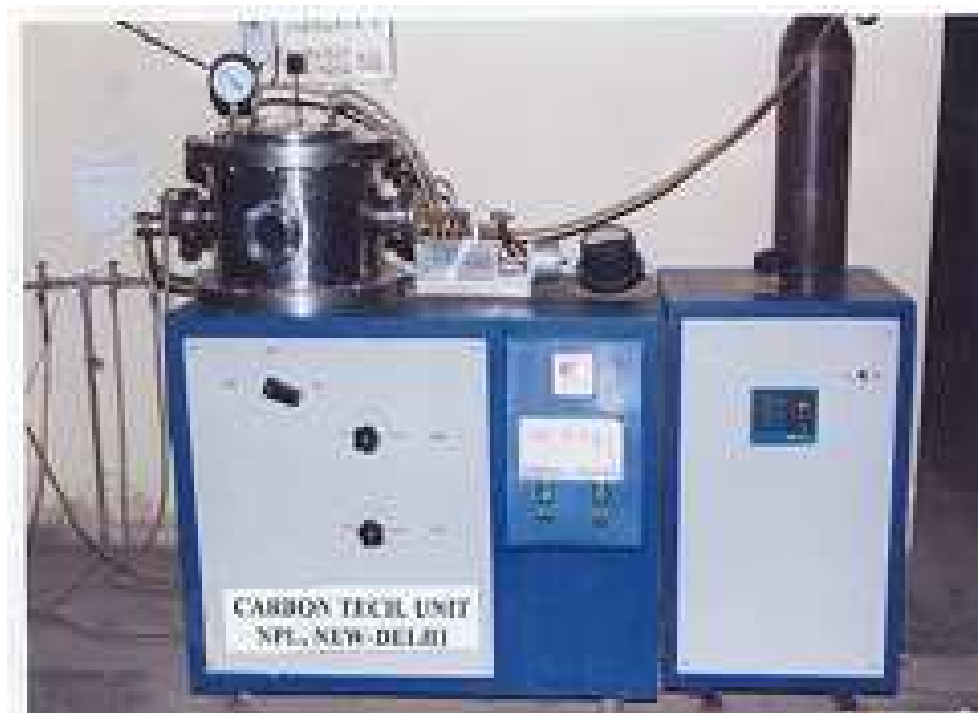
Figure 5.1.1: Set-up for producing carbon nanotubes by dc electric arc discharge
