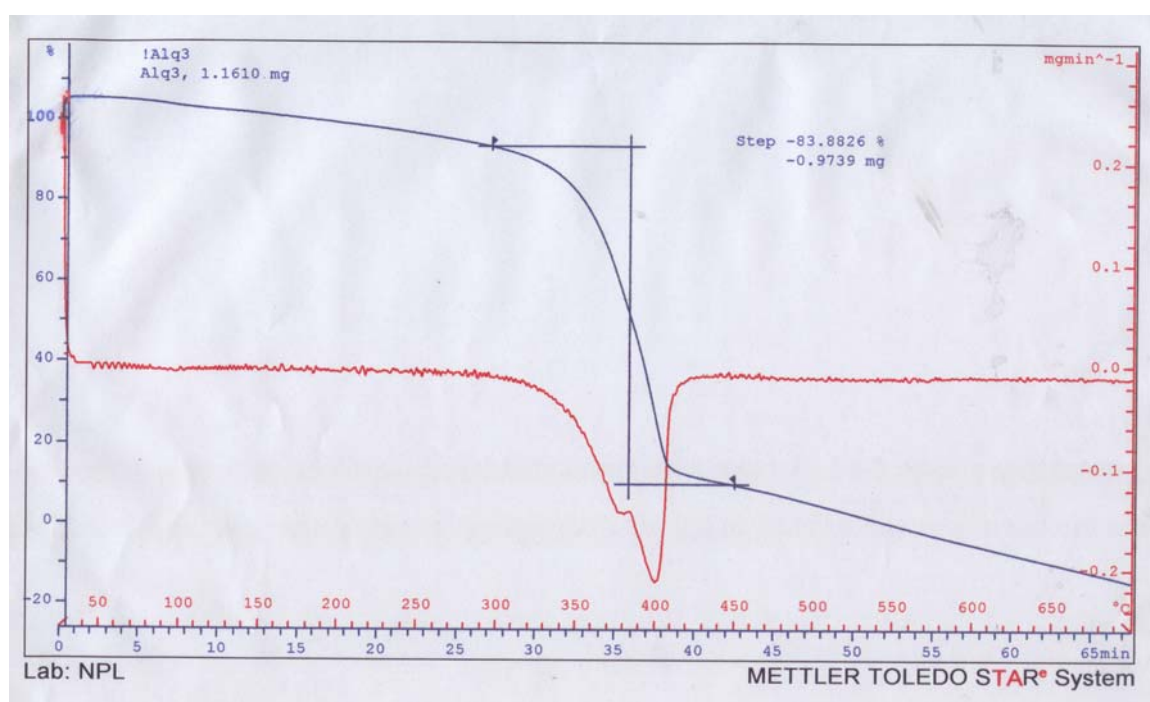
Figure 4.3 Thermogravimetric Analysis of Alq 3
