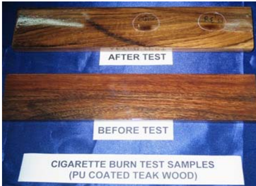
Fig 18 PU coated teak wood samples for cigarette burn resistance
