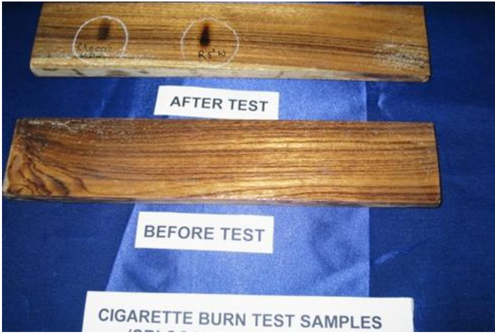
Fig 17ABC coated teak wood samples for cigarette burn resistance
