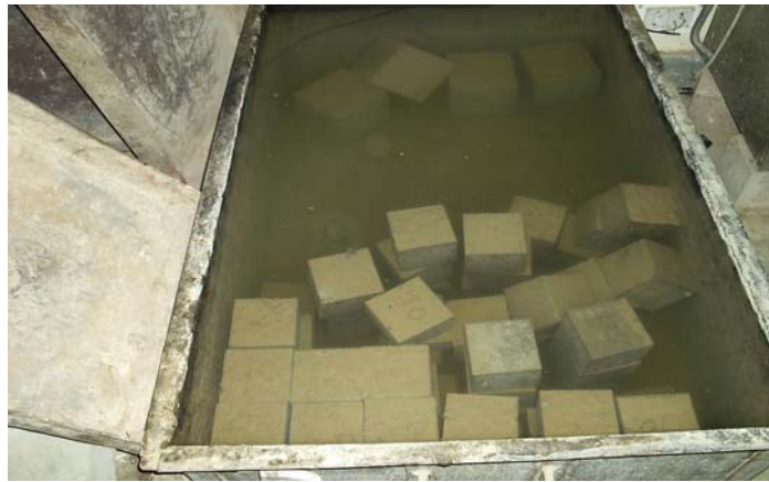
Curing of cubes
