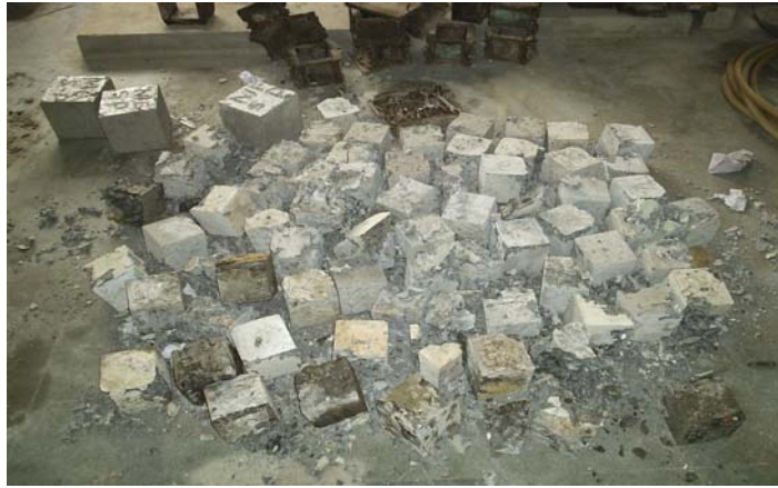
Cubes after measuring compressive strength
