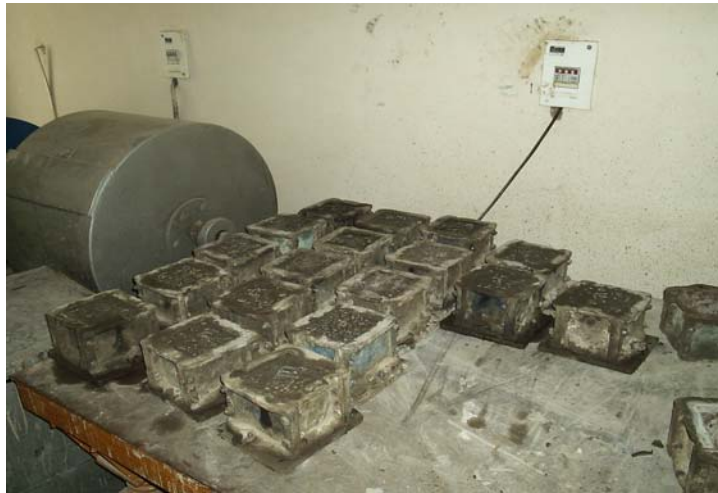
Casting of cubes
