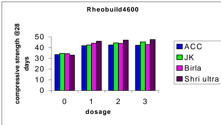
Figure 90: Variation of strength with dosage for M30 concrete
