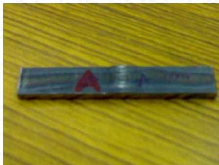
Fig 4.16: Sample (A, B&C) test pieces for tensile, micro and bend test
