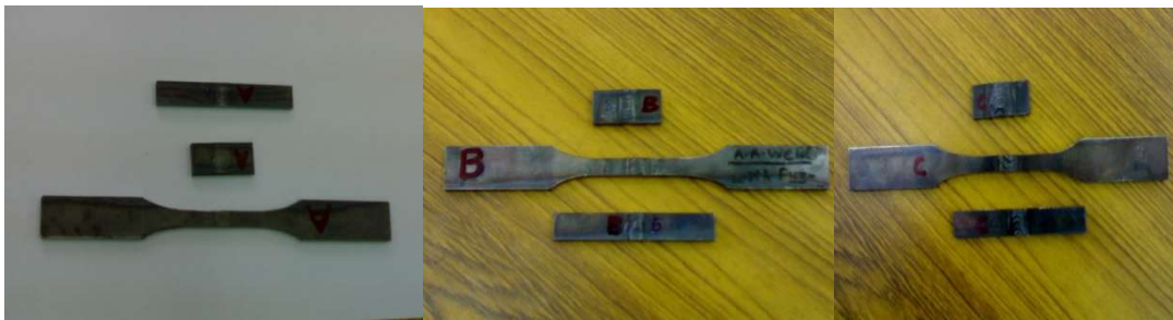
Fig 4.16: Sample (A, B&C) test pieces for tensile, micro and bend test
