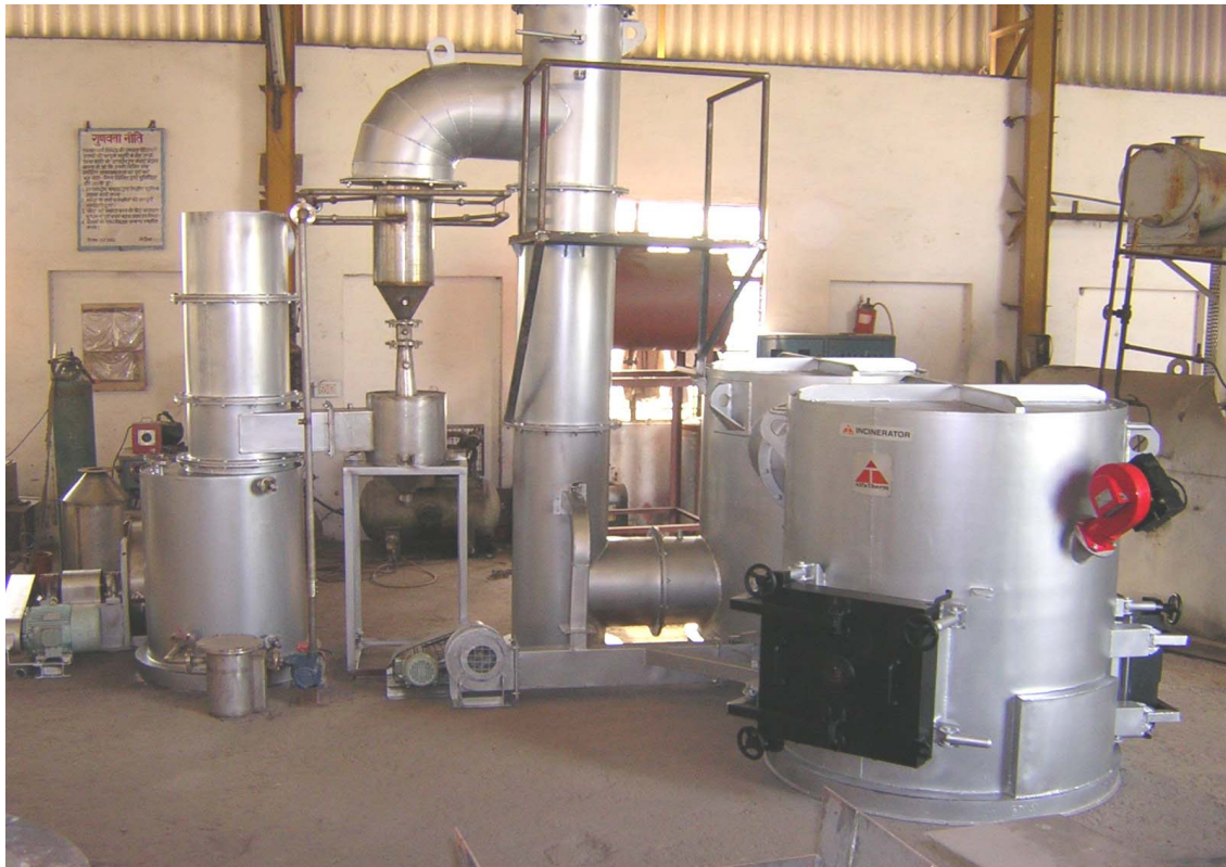
Figure 4.1 Incinerators complete with pollution control equipments
