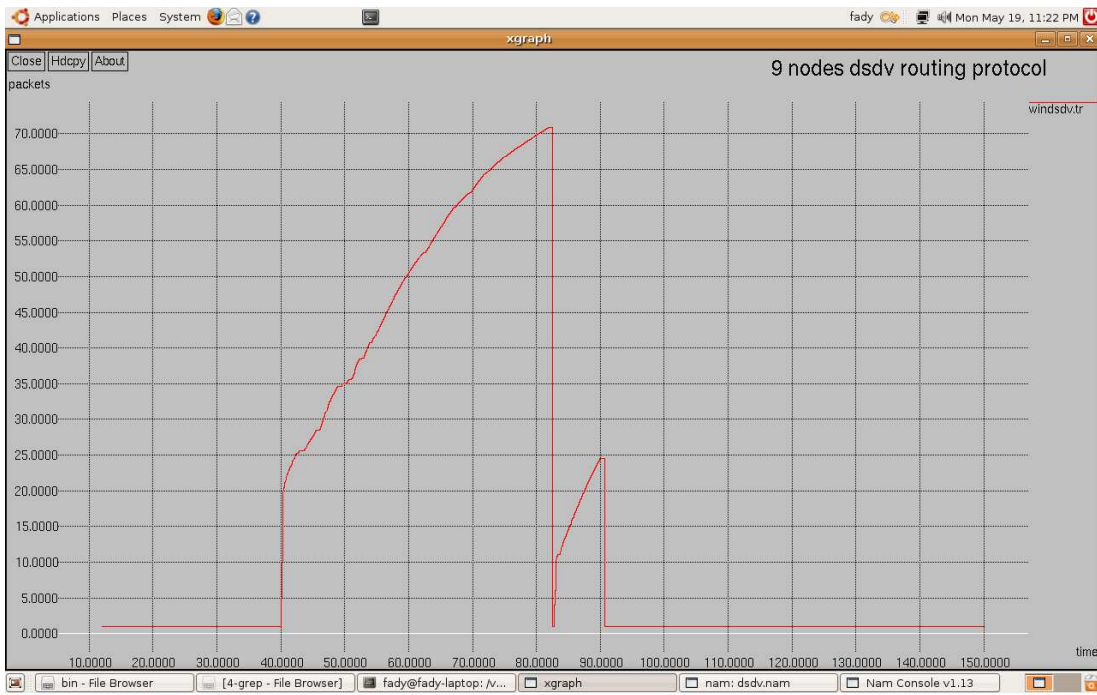
Figure 5.21 TCP window size in a nine nodes scenario with DSDV routing protocol
