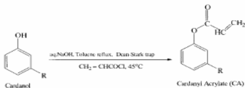
Scheme 2.1.3.2. Preparation of cardanyl acrylate
