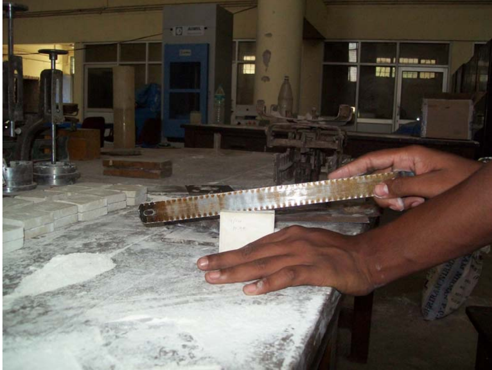
Fig 3.4 Preparation of Type II Joint Surface
