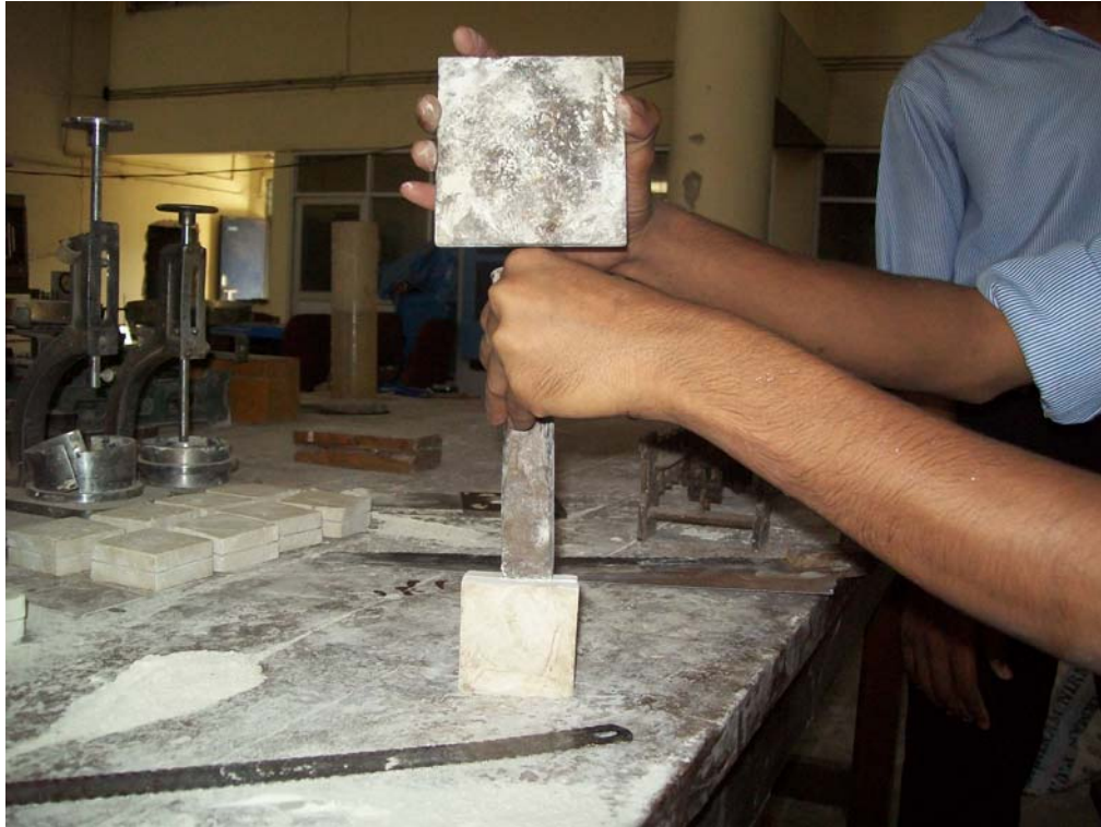
Fig 3.2 Preparation of Type I Joint Surface
