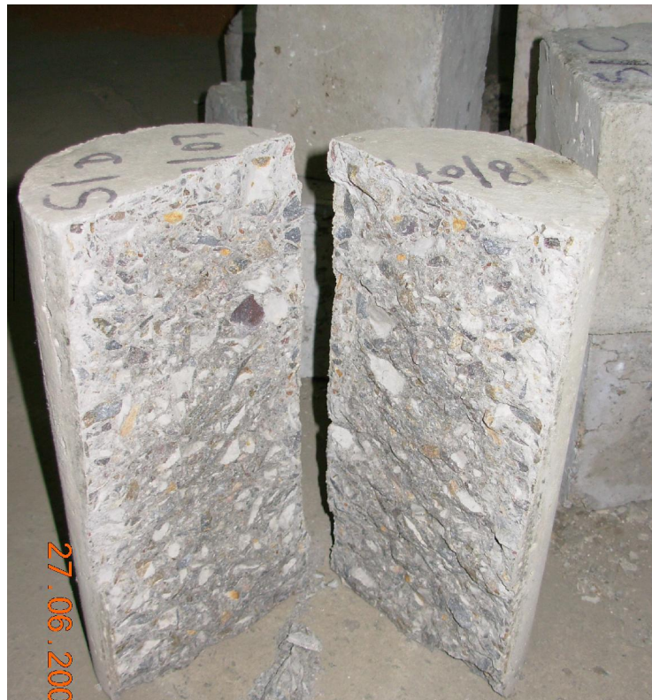
Fig 5.4 Split surface of cylinder
