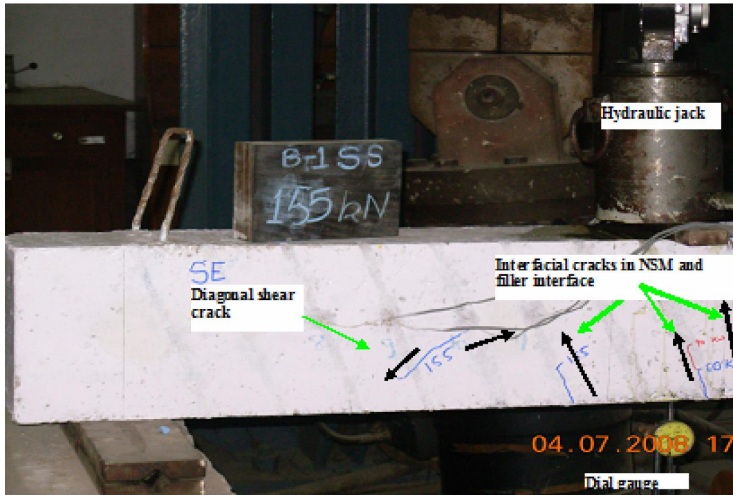
Fig 7.17 Test B1-SS crack pattern at 155 kN (Face SE)
