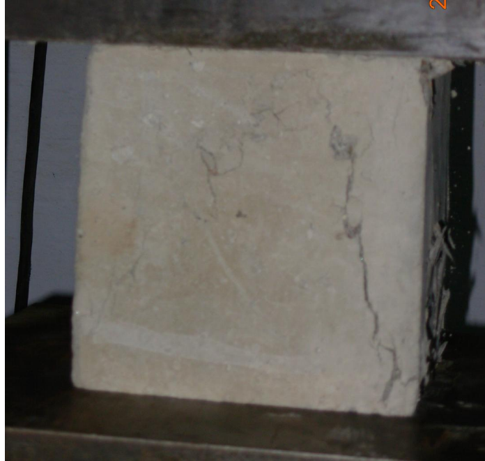
Fig. 5.2 Compressive failure of cube
