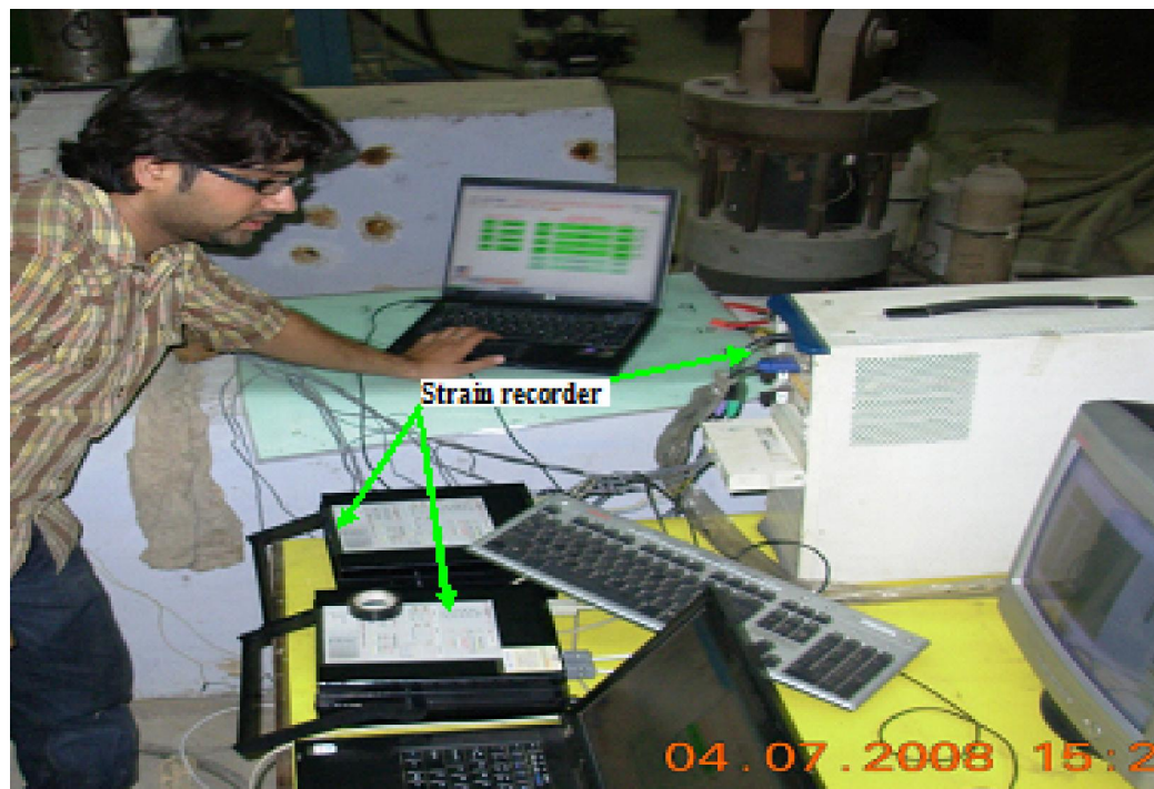
Fig 7.14 Arrangement for strain recording
