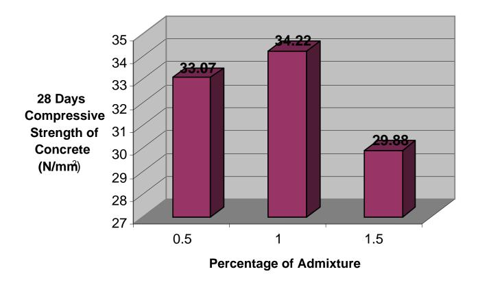
**28** Days compressive strength of concrete (N/mm<sup>2</sup>)
