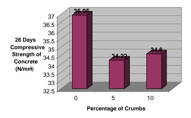
■ 28 Days compressive strength of Concrete (N/mm<sup>2</sup>)
