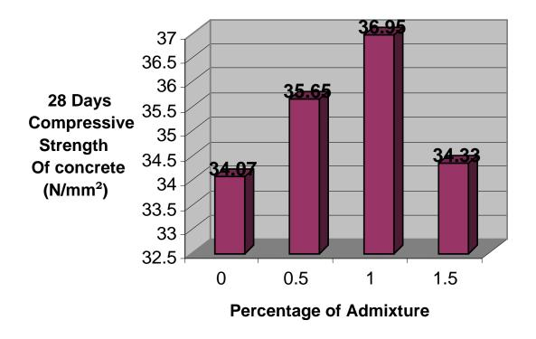
**28** Days compressive strength of concrete (N/mm<sup>2</sup>)
