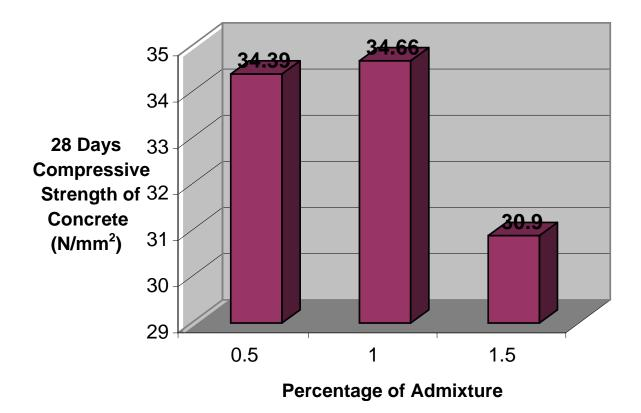
■ 28 Days compressive strength of Concrete (N/mm<sup>2</sup>)
