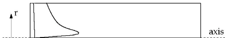
Typical Radial Distribution of w in a Free Vortex
