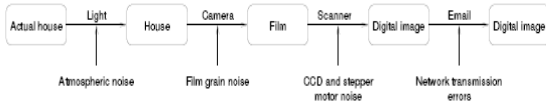
Figure 3: Noise may be introduced at each step in the acquisition process
