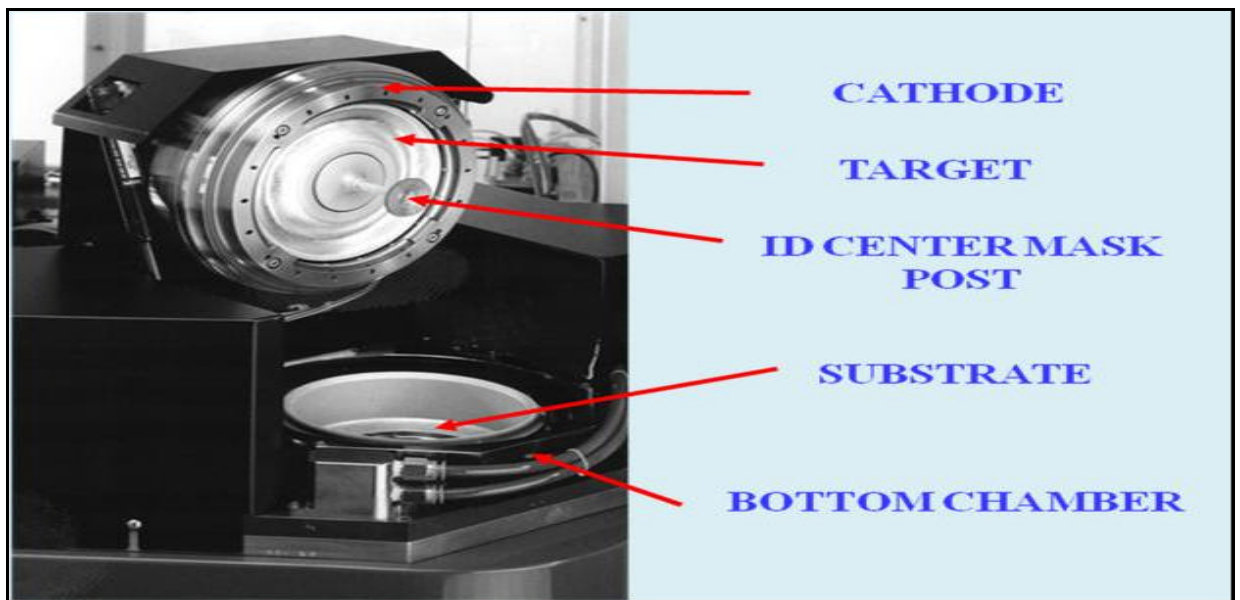
Fig 51 Uni-jet metallizer showing the sputter chamber
