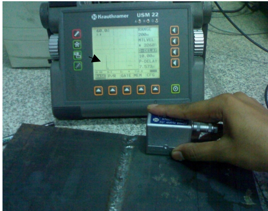
Figure 8.3h, 3 rd Defect Echo on CRT Screen
