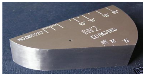
Figure 5.3b, IIW (V2) Calibration Block
