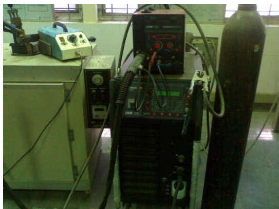
Figure 8.1a, Synergic MIG Welding Machine Setup
