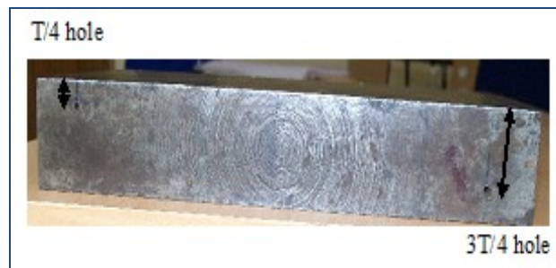
Figure 7.4a, Reference Block with Drilled Hole
