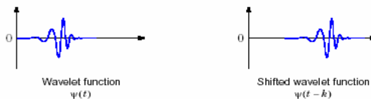
Figure 3.5 Shifting of a signal
