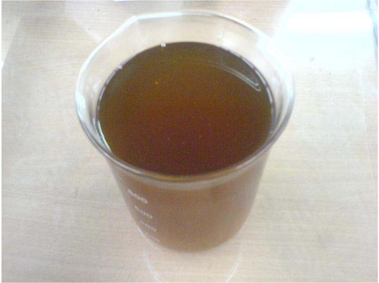
Figure 3.7 Biodiesel prepared from thumba oil.
