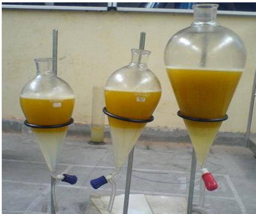
Figure 3.6 washing process of biodiesel
