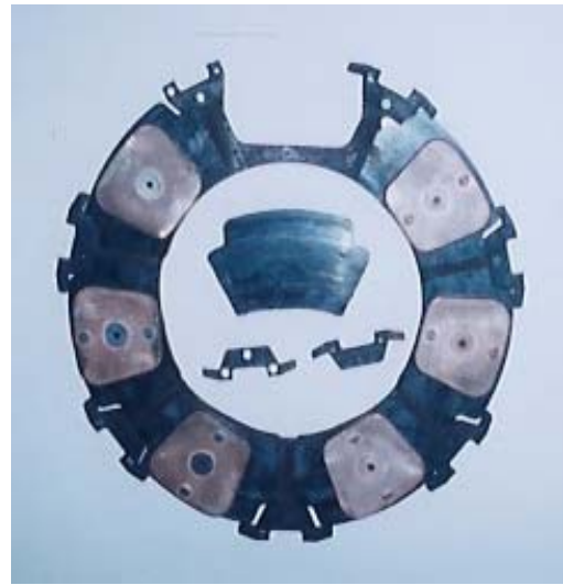
Fig.12 Rotor plate after removing one segment Friction plates are placed above the plate
