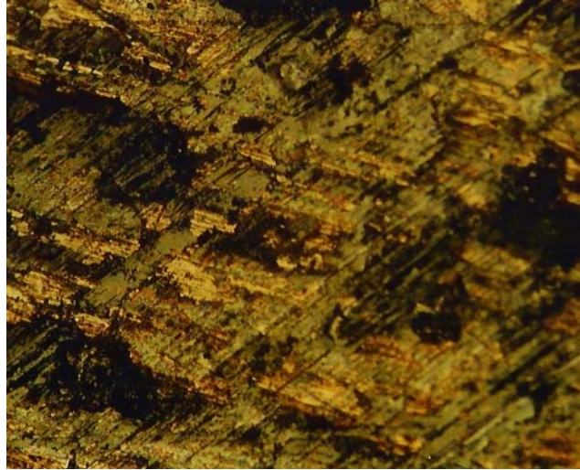
Fig.20 Surface texture (300 x magnification) of sample-III after test (Load=10 N, Track dia=32 mm, rpm=60, time=1 hour)
