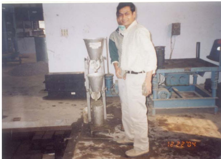
Fig: 2 Compaction Factor test in progress
