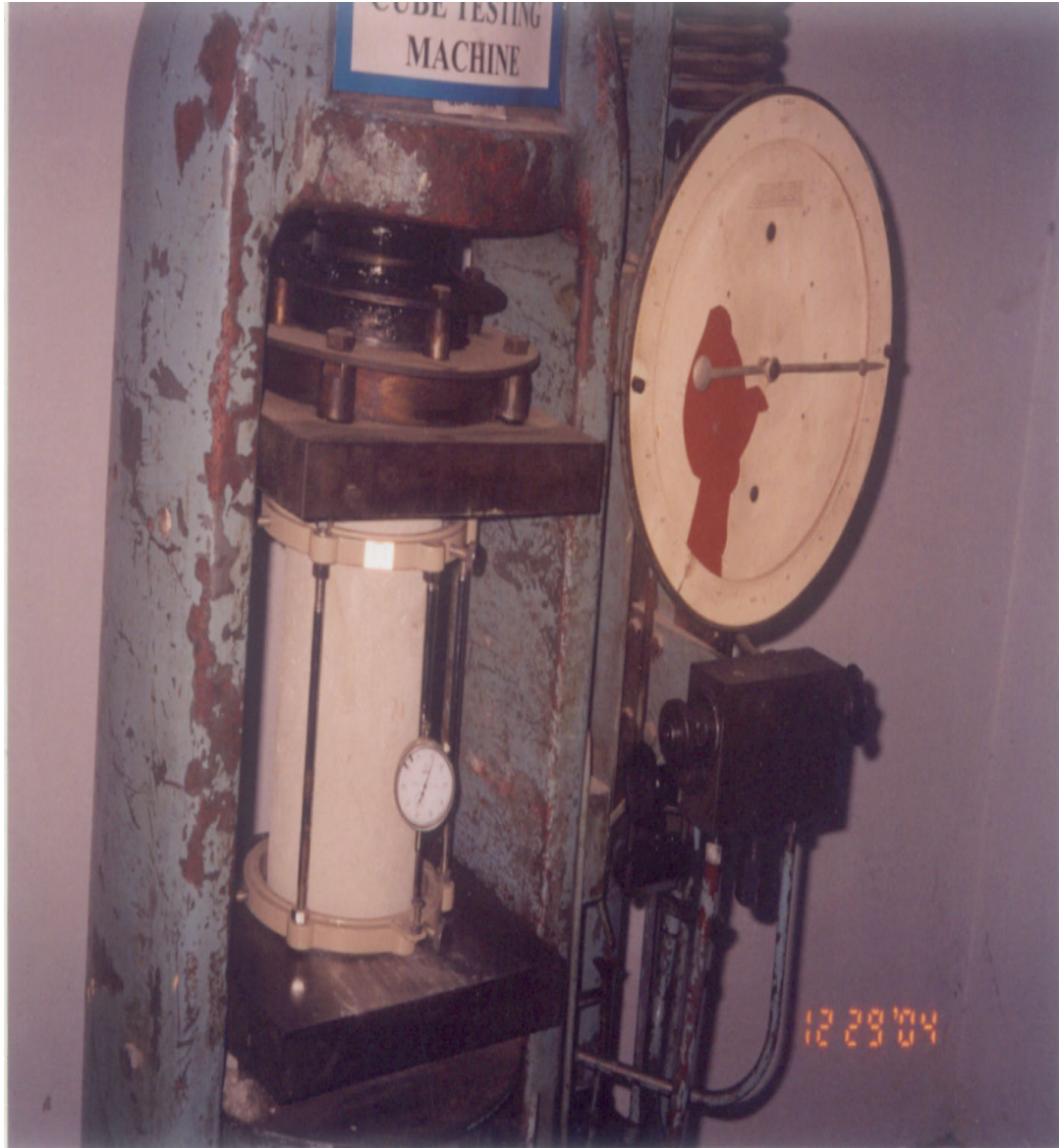
Fig: 7 Modulus of Elasticity test in progress
