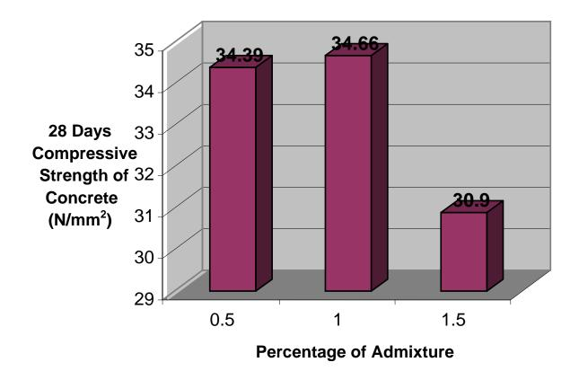
■ 28 Days compressive strength of Concrete (N/mm²)
