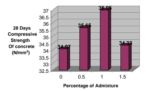
■ 28 Days compressive strength of concrete (N/mm²)
