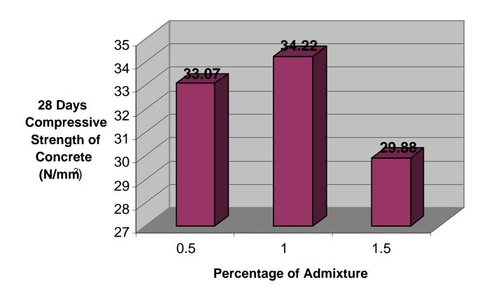
■ 28 Days compressive strength of concrete (N/mm²)
